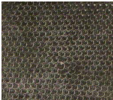
Fig. 11. Bubble model of impurity atom in a crystal [4]
