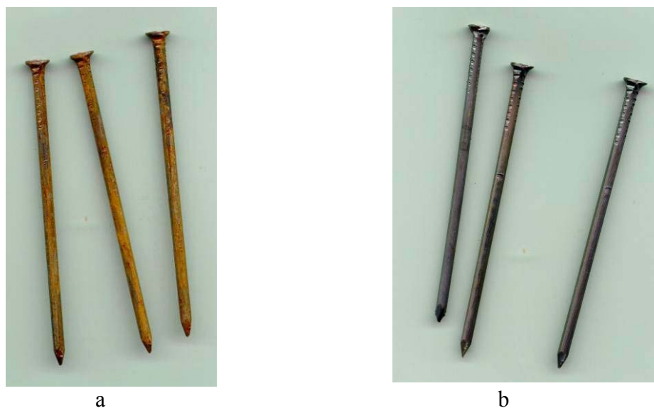
Fig. 25. Exterior of the samples after atmospheric tests, a – original samples; b – treated samples [2, 40]
